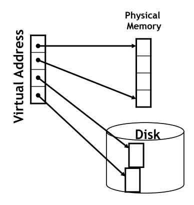
A virtual address can be mapped to either physical memory or disk.
