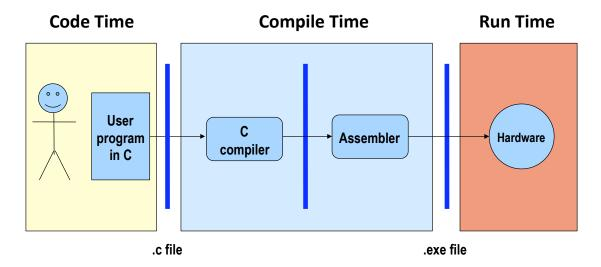
Note: The compiler and assembler are just programs, developed using this same process.
