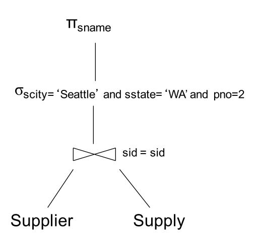
Supplier(<u>sid</u>, sname, scity, sstate) Supply(<u>sid</u>, <u>pno</u>, quantity)
