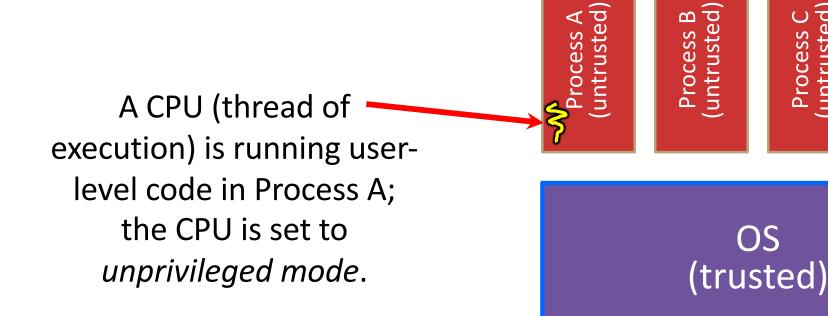
Code in Process A invokes a system call; the hardware then sets the CPU to *privileged mode* and traps into the OS, which invokes the appropriate system call handler.
