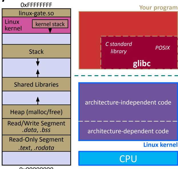
**OxFFFFFFF** Your program linux-gate.so Process is executing your Linux kernel stack program code kernel C standard **POSIX** library Stack SP [ glibc **Shared Libraries** architecture-independent code Heap (malloc/free) Read/Write Segment .data, .bss architecture-dependent code Read-Only Segment **Linux kernel** .text, .rodata **CPU** unpriv 0x0000000
