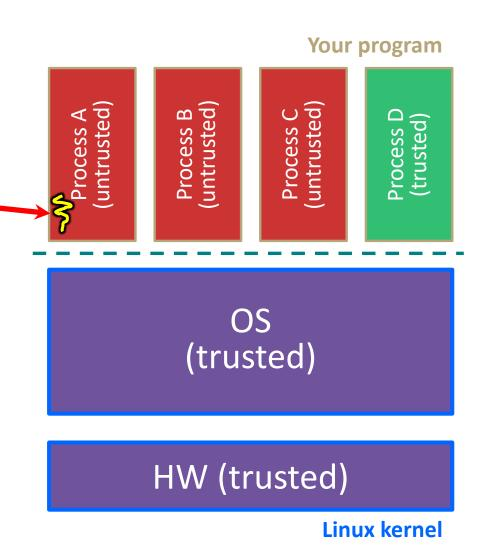
Code in Process A invokes a system call; the hardware then sets the CPU to privileged mode and traps into the OS, which invokes the appropriate system call handler.
