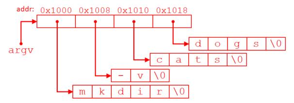
argv is the second parameter, so its value is stored in <code>%rsi</code> and does not take up space in memory. The character arrays have unknown/unspecified addresses that are stored in the entries of <code>argv</code>. Each character of the command-line arguments takes up 1 byte of memory and the elements of each character array have consecutive addresses, though the arrays are likely not contiguous to each other.
