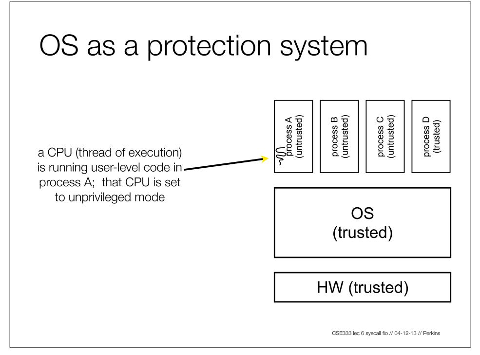
code in process A invokes a system call; the hardware then sets the CPU to privileged mode and traps into the OS, which invokes the appropriate system call handler
