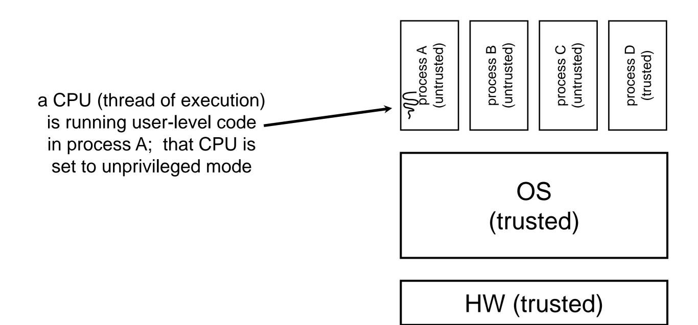
code in process A invokes a system call; the hardware then sets the CPU to privileged mode and traps into the OS, which invokes the appropriate system call handler
