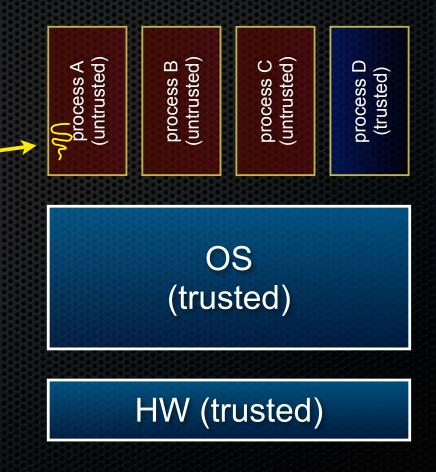
code in process A invokes a system call; the hardware then sets the CPU to privileged mode and traps into the OS, which invokes the appropriate system call handler
