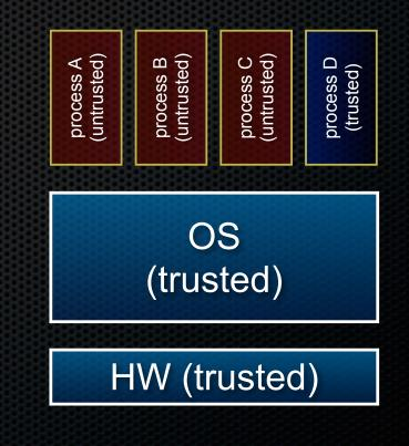
a CPU (thread of execution) is running user-level code inprocess A; that CPU is set to unprivileged mode
