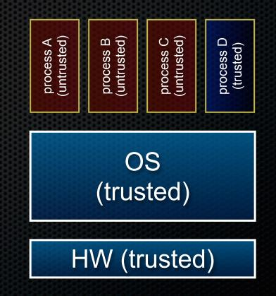
a CPU (thread of execution) is running user-level code inprocess A; that CPU is set to unprivileged mode
