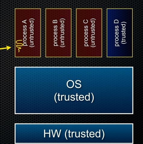
code in process A invokes a system call; the hardware then sets the CPU to privileged mode and traps into the OS, which invokes the appropriate system call handler
