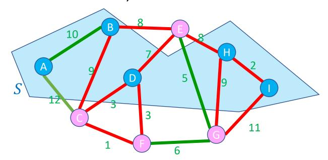
Edge  $(v_1, v_2) \in E$  crosses a cut if  $v_1 \in S$  and  $v_2 \in V - S$  (or opposite), e.g. (A, C)
