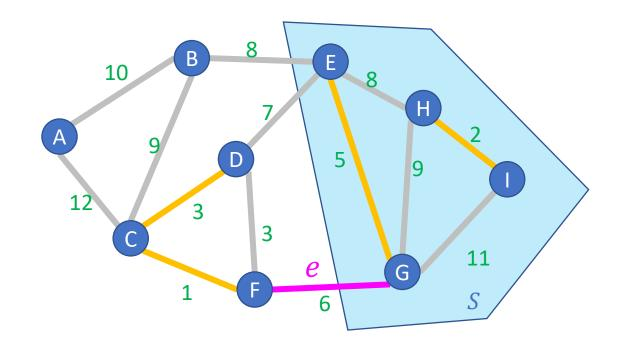
Keep edges in a Disjoint-set data structure (very fancy)  $O(E \log V)$
