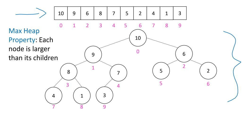
Remove the Max element (i.e. the root) from the Heap: replace with last element, call percolateDown(root)
