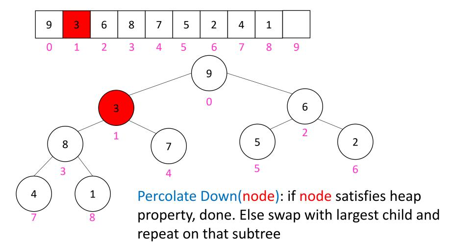
Remove the Max element (i.e. the root) from the Heap: replace with last element, call percolateDown(root)
