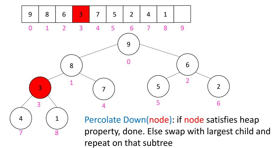
Remove the Max element (i.e. the root) from the Heap: replace with last element, call percolateDown(root)
