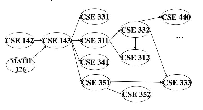
Node: 126 142 143 311 312 331 332 333 341 351 352 440 Removed? x x x x x x x x In-degree: 0 0 2 1 2 1 1 2 1 1 1 1
