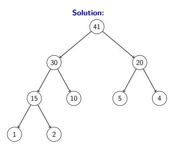
(b) Re-order the numbers so that if you were to insert them into a heap again, (1) the result would be an identical heap, and (2) the number of comparisons is minimal.
