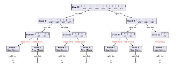
Once your divide-and-conquer tree gets to a certain depth with respect to cutoff, you should switch to a sequential algorithm. (Namely, minimax.) Furthermore, as above, you will be doing a divide-and-conquer algorithm; so, there will be a second cutoff, divideCutoff, which will tell the algorithm when to stop dividing nodes.
