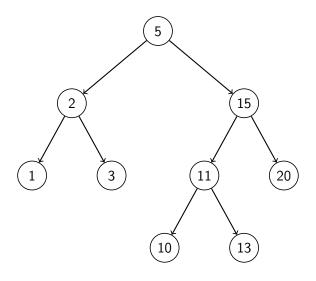
NOTE: We will need to do a single rotation when inserting the 1 and the 20, and a double rotation when inserting the 3 (10-2-5 kink) and the 11 (10-13-11 kink).
