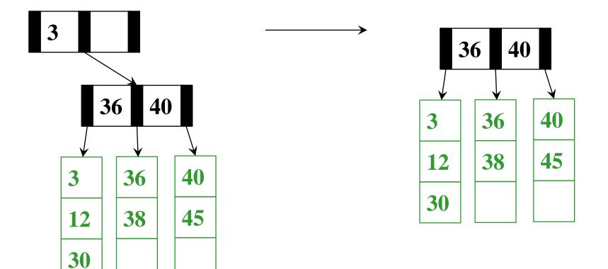
Which causes an underflow in root; replace root
