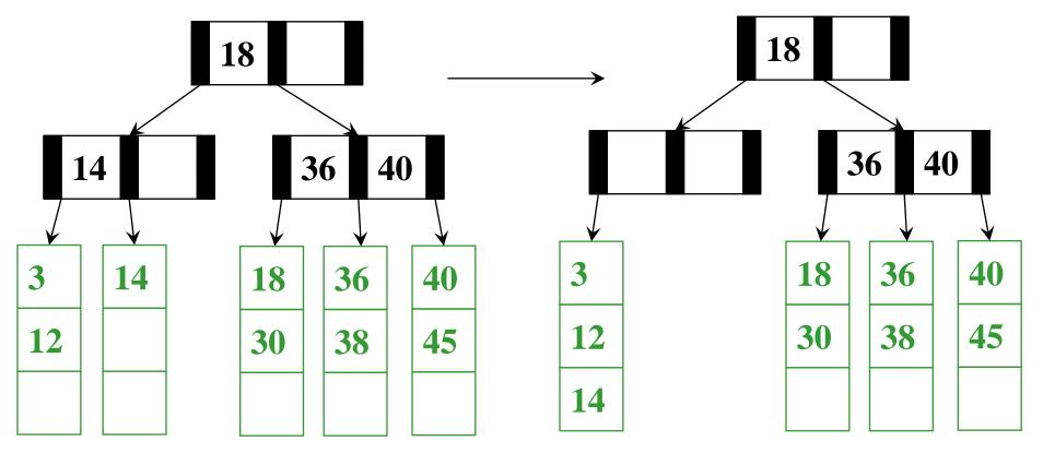
Merge the two nodes together. This causes underflow in the parent
