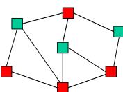
Input: A graph (V,E) and a number m Output: A subset S of V such that for every edge (u,v) in E, at least one of u or v is in S and |S|=m (if such an S exists)
