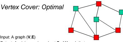
Input: A graph (V,E) Output: A minimum size subset **S** of **V** such that for every edge (u,v) in **E**, at least one of u or v is in **S**
