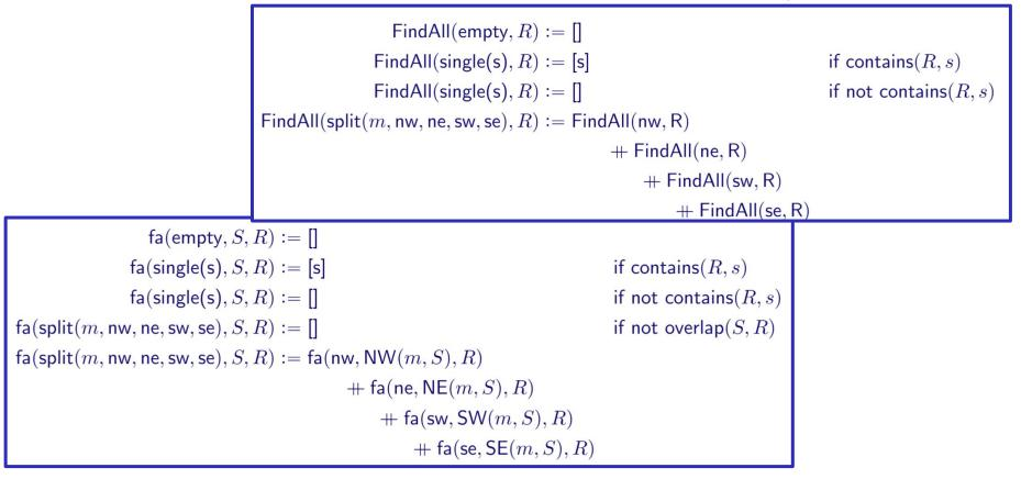
**Introduction:** Define P(T) to be the claim that, if region S contains all locations in tree T, then fa(T, S, R) = FindAll(T, R). We will prove this holds by structural induction **Base Cases (T is empty or single):** Note that if S does not contain s, the P is vacuously true
