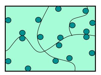
Small subdomains at the edges of the "main" subdomains have a high probability of revealing many common errors
