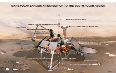
Legs deployed → Sensor signal falsely indicated that the craft had touched down (130 feet above the surface)
