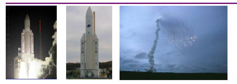
The rocket self-destructed 37 seconds after launch Reason: A control software bug that went undetected Conversion from 64-bit floating point to 16-bit signed integer value had caused an exception The floating point number was larger than 32767 (max 16-bit signed integer)
