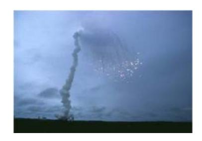
The rocket self-destructed 37 seconds after launch Reason: A control software bug that went undetected
