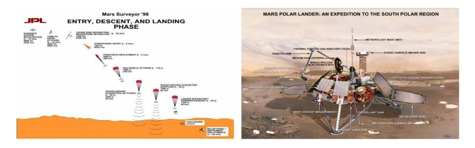
Legs deployed → Sensor signal falsely indicated that the craft had touched down (130 feet above the surface) Then the descent engines shut down prematurely The error was traced to a single bad line of software code. Why didn't they blame the sensor? NASA investigation panel blames for the lander failure,
