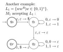
This machine is almost exactly like M above, except for the transition between states 1 and 2. Essentially, we are constantly checking if the "second half" of the input is the reverse of the first half. Next time, we'll see how exactly the machine behaves on some input.
