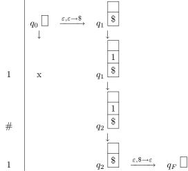
Since one branch is in an accept state after reading the input string, the machine accepts the input string.
