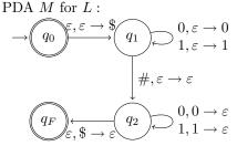
In this PDA,  $q_1$  is the state for "pushing" w and state  $q_2$  is the state for "popping" w and matching it to  $w^R$ .
