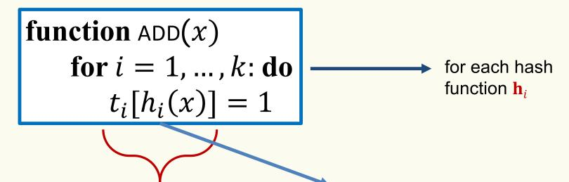
Index into *i*-th bit-vector, at index produced by hash function and set to 1
