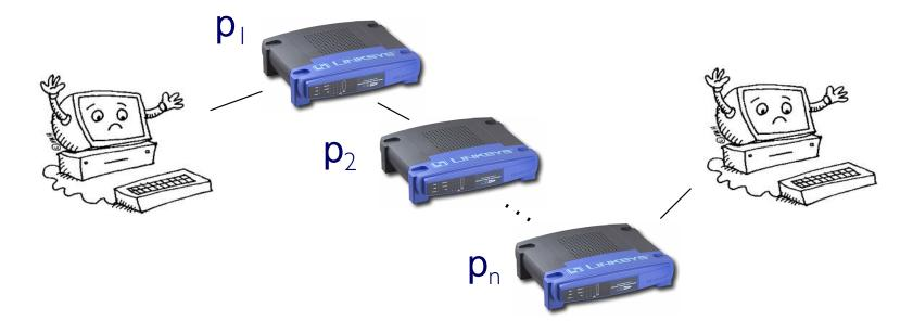
n routers, i<sup>th</sup> has probability p<sub>i</sub> of failing, independently P(there is functional path) = P(no routers fail)
