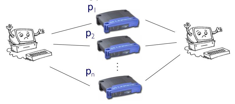
n routers, i<sup>th</sup> has probability  $p_i$  of failing, independently P(there is functional path) = I - P(all routers fail)
