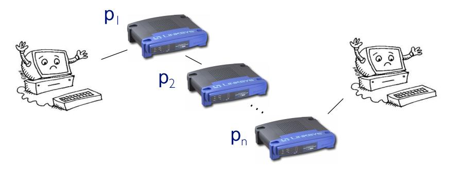
n routers, i<sup>th</sup> has probability  $p_i$  of failing, independently  $P(\text{there is functional path}) = P(\text{no routers fail}) = (I - p_1)(I - p_2) \cdots (I - p_n)$
