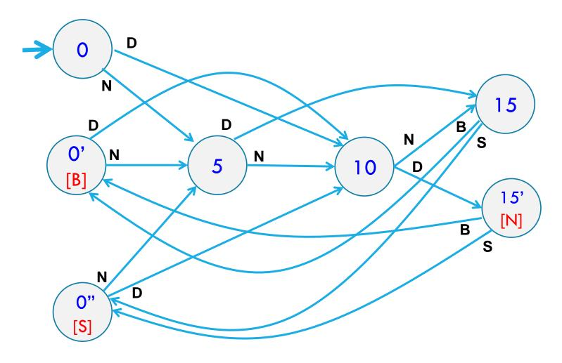
Adding output to states: N – Nickel, S – Snickers, B – Butterfinger
