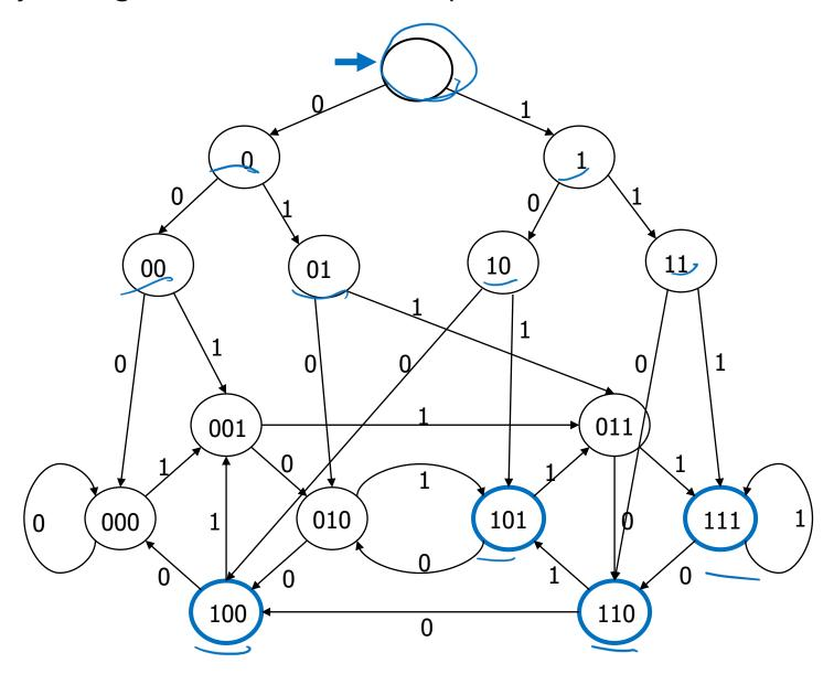
The set of binary strings with a 1 in the 3<sup>rd</sup> position from the end
