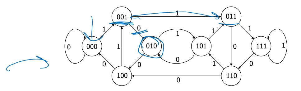
The set of binary strings with a 1 in the 3<sup>rd</sup> position from the end
