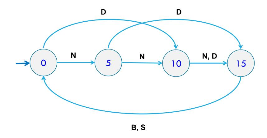
Basic transitions on **N** (nickel), **D** (dime), **B** (butterfinger), **S** (snickers)
