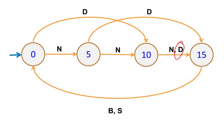
Basic transitions on **N** (nickel), **D** (dime), **B** (butterfinger), **S** (snickers)
