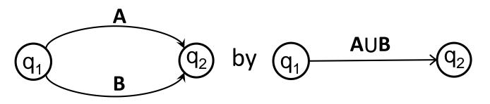
**Rule 2**: Eliminate non-start/final state q<sub>3</sub> by replacing all
