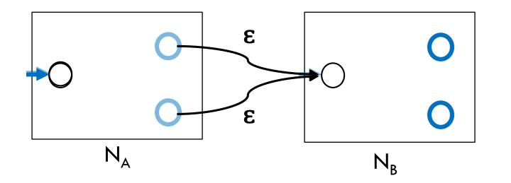
String x that matches AB can divide into yzwhere y matches A, z matches B. NFA can run as  $N_A$  would on y take  $\varepsilon$ -transition, then run as  $N_B$  would on z so accepted by N String x that is accepted? N must run in  $N_A$  take  $\varepsilon$ -transition, then run in  $N_B$  until acceptance. Substring read in  $N_A$  must match A. Substring read in  $N_B$  must match B (by IH) so string matches AB.
