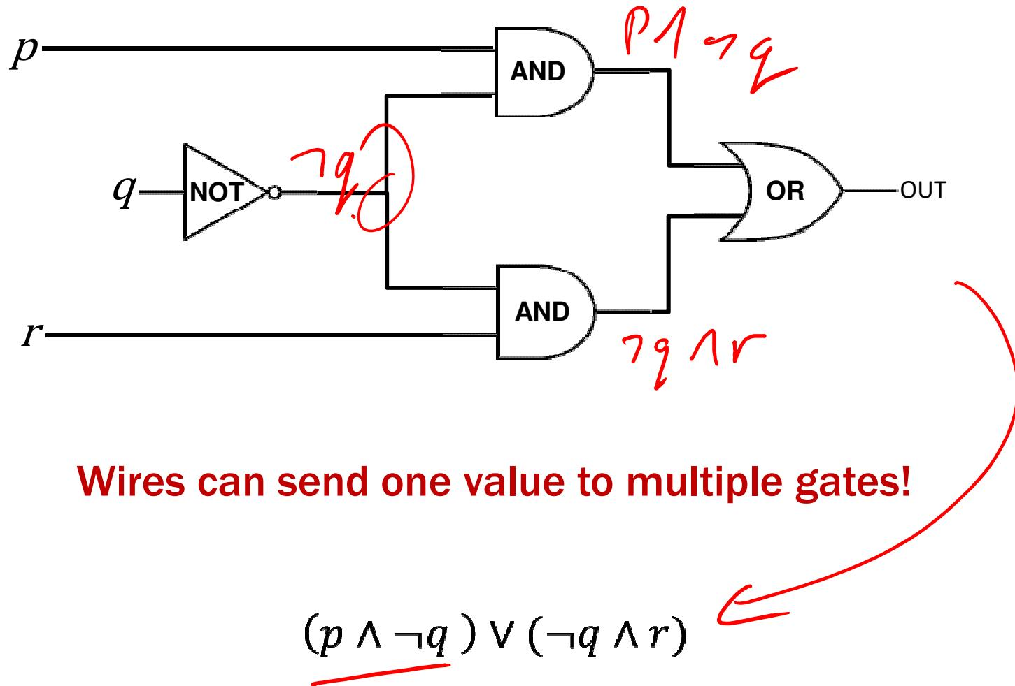
Wires can send one value to multiple gates!
