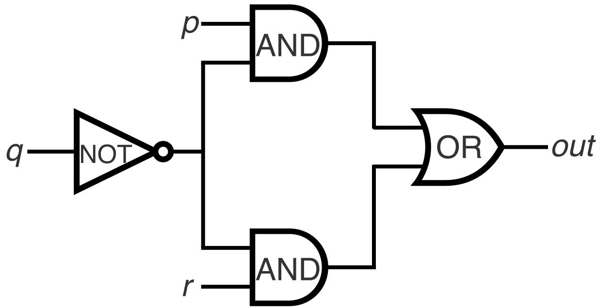
Wires can send one value to multiple gates.
