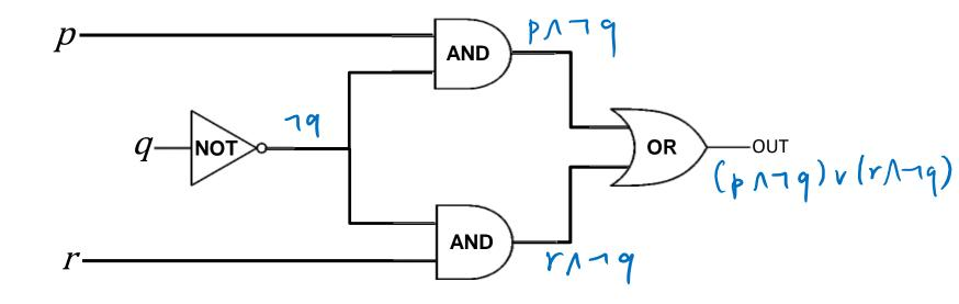
Wires can send one value to multiple gates!
