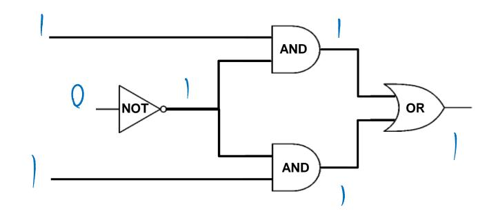
Wires can send one value to multiple gates!
