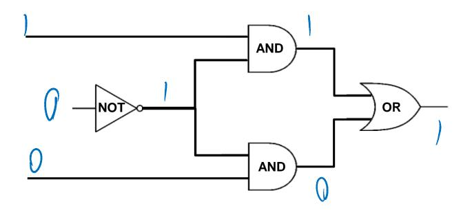
Wires can send one value to multiple gates!
