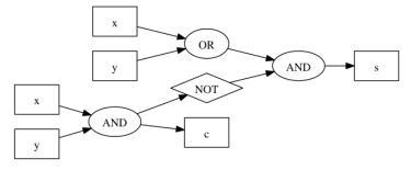
**Note:** All of the above was done with just AND, OR and NOT gates. If we allow XOR gates, then we can have a much simpler circuit with just 2 gates (1 XOR, 1 AND):
