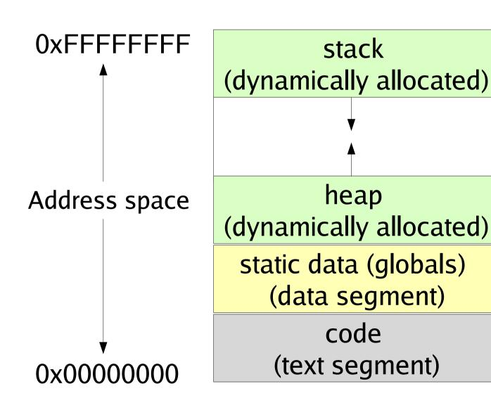
Address space is just array of 8-bit bytes
