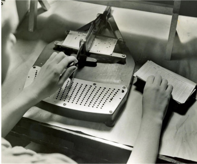
A pantograph used to create punch cards
