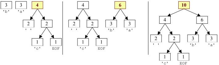
Notice that the nodes with low frequencies end up far down in the tree, and nodes with high frequencies end up near the root of the tree. This structure can be used to create an efficient encoding. The Huffman code is derived from this tree by thinking of each left branch as a bit value of 0 and each right branch as a bit value of 1:
