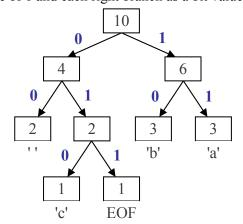
The code for each character can be determined by traversing the tree. To reach ' ' we go left twice from the root, so the code for ' c' is 00. The code for 'c' is 010, the code for EOF is 011, the code for 'b' is 10 and the code for 'a' is 11. By traversing the tree, we can produce a map from characters to their binary representations. For this tree, it would be: { ' '=00, 'a'=11, 'b'=10, 'c'=010, EOF=011}
