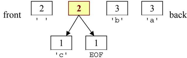
This process is repeated until the queue contains only one binary tree node with all the others as its children. This will be the root of our finished Huffman tree. The following diagram shows this process:
