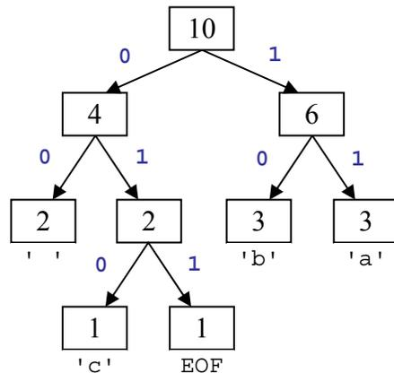
The code for each character can be determined by traversing the tree. To reach ' ' we go left twice from the root, so the code for ' ' is 00. The code for 'c' is 010, the code for EOF is 011, the code for 'b' is 10 and the code for 'a' is 11. By traversing the tree, we can produce a map from characters to their binary representations. For this tree, it would be:
