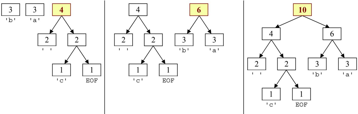
Notice that the nodes with low frequencies end up far down in the tree, and nodes with high frequencies end up near the root of the tree. This structure can be used to create an efficient encoding. The Huffman code is derived from this tree by thinking of each left branch as a bit value of 0 and each right branch as a bit value of 1:
