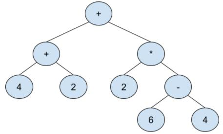
Running the method calculate() with this tree would return the integer 10. Assume that the given tree will have at least 3 nodes (enough for one operation) and will always be in correct format (mathematically correct)
