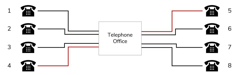
• The telephone office makes connections based on how you dial the keypad.
