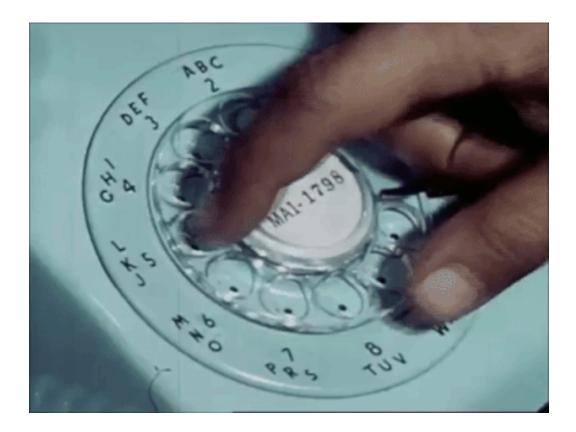
**Pulse Dialing:** Rotating the dial to a certain number sends that number of short pulses down the telephone line by disconnecting and reconnecting the hook switch.
