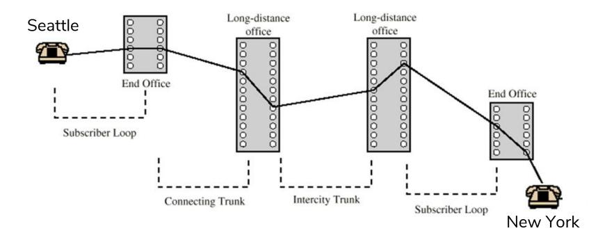
Long distance calls travel through multiple offices that need to find unused lines through which connections can be made.
