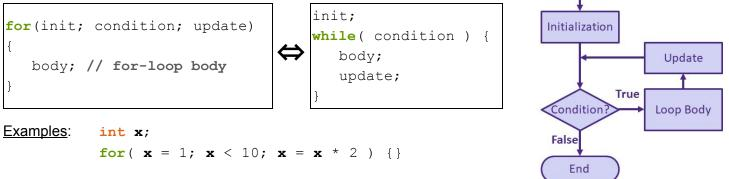
This (empty body!) for-loop is equivalent to the while-loop example: we're able to eliminate the entire body of the loop because it's now executed as the update statement!
