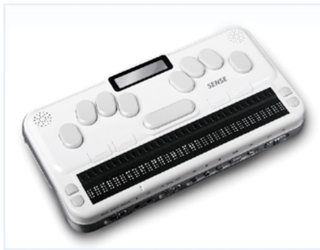
Refreshable Braille Display, WiFi Enabled
