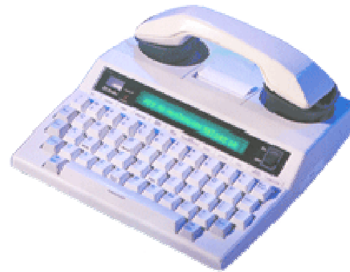
Modern TTY with built-in acoustic modem
