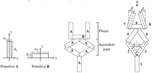
Assume that  $\alpha$  and  $\beta$  can take values in the range  $[0, 90^{\circ}]$ . Also assume that all parts use primitive **A**, except for part **6**, which uses primitive **B**. The model on the left shows the primitives used, the model on the right shows the enumeration (naming) of the parts.
