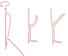
Idea: rotate a 2D **profile curve** around an axis.
