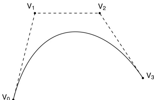
Compare total length of control polygon to length of line connecting endpoints:
